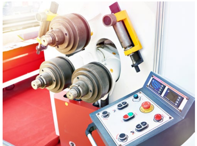
Traditional machine designs include safety-related switches and emergency stops on a stationary panel. Hydraulic profile bender image: Ryzhov Sergey • Dreamstime
